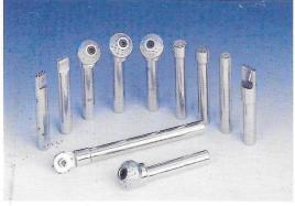
Balaji Single Point Diamond Dresser's are made of selected diamonds, Mounted in a matrix. Only one cutting edge is presented to the grinding wheel. Diamonds for Single Point Dressing Tools are selected for their structural strength, number of points, degrees of sharpness, and lack of determental flaws. The proper selection of size and quality appropriate for a given application required qualified judgement.
