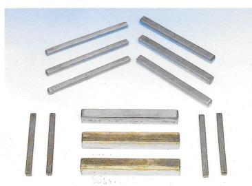
Diamond/CBN hones with their economically longer life, have contributed in no small measures to this rapid development. Diamond/CBN honing has proved in particular suitable means of honing mass - production in cast - iron parts, steel components, like honing gear bores, connecting rod, which major application in the transport industry.
