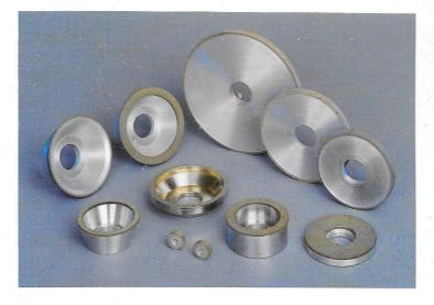
**Balaji** Diamond Wheels are of superior quality and available in Resin, Metal and Electrometallic bonds. They are used for grinding carbides, glass, ceramics, ferrites and other hard and abrasive materials. These are available in diameters ranging from 10.0 mm to 300 mm. Bond type, grit size and concentration are selected to ensure maximum wheel performance according to the application.
