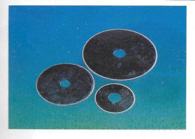
Continuous rim type diamond saw blades are used for cutting various materials such as tungsten carbide, ceramics, glass, ferrites, synthetic stones and other construction materials such as glazed tiles etc. available in various sizes from 75 to 300 mm dia. These cut-off wheels can also be used for cutting high density carbons, fibre glass, glass rein forced plastics, hard rubbers and hard plastics.
