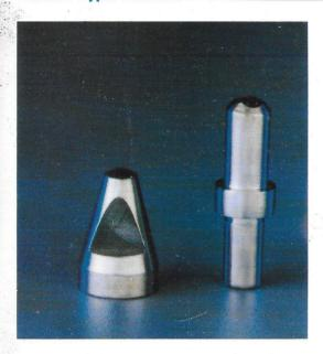
A superior quality clean "GEM" quality Diamond is super lapped to a square pyramid with an apex angle of 136 Degrees, to provide the highest standards of precision and performance.
