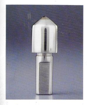
An exceptionally fine clean Octahedron diamond is super lapped to an exact angle of 120 degrees with incredible MICROFINISH, to provide the highest standards of precision and performance.
